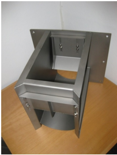
Fig. 5.3 Double baffle controller
