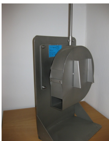
Fig. 6.5 Vertical centrifugal valve
